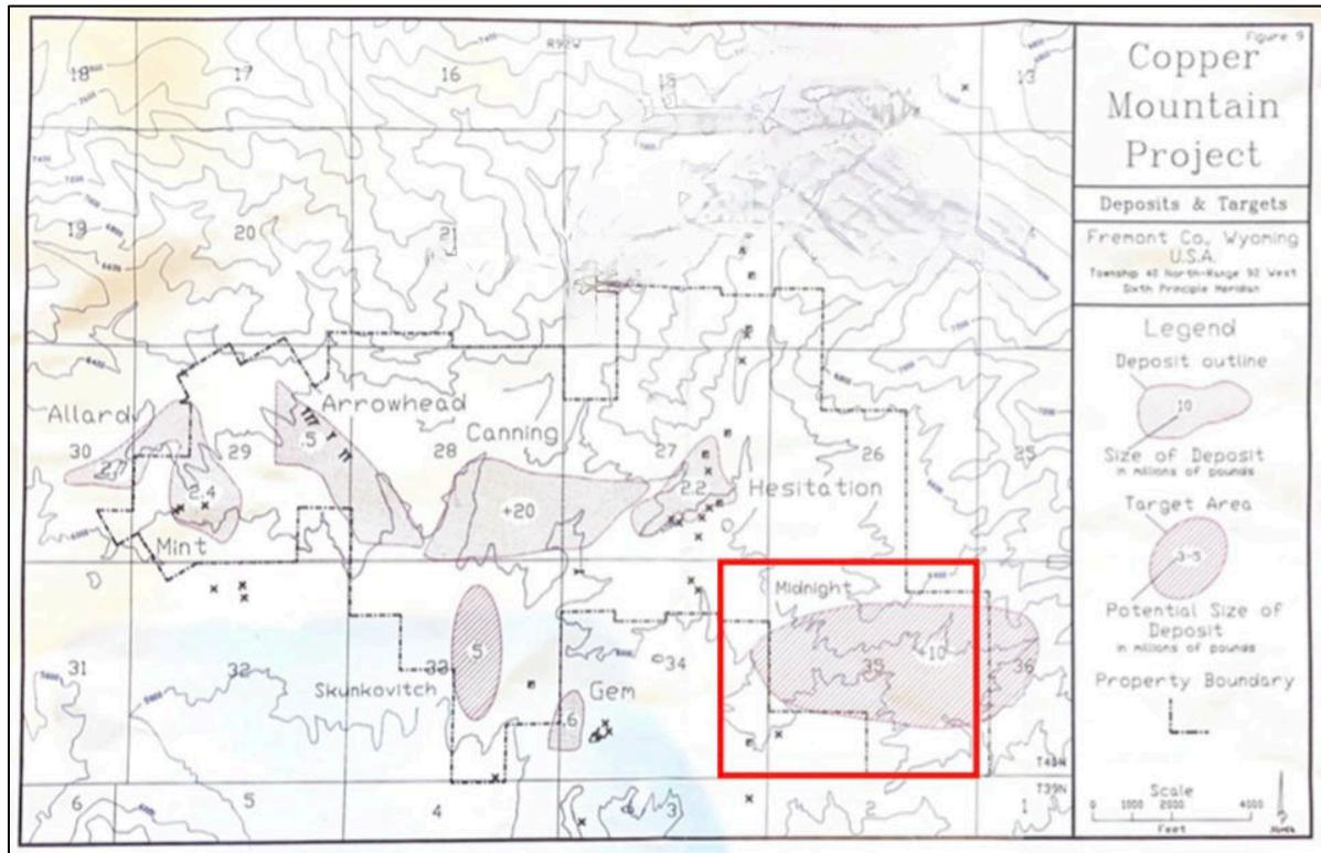
Figure 2: Midnight claims (red rectangle) on a map from a 1991 Anaconda report indicating the Midnight Prospect, which potentially contains up to 10 Mlbs  $eU_3O_8$ . (Confidential information redacted).
